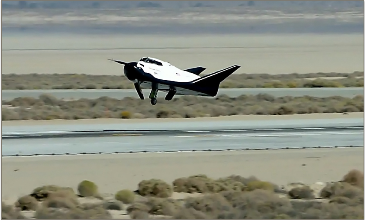
The Dream Chaser engineering test article coming in for an autonomous landing during October 2013 at Edwards Air Force Base, Calif. As the image clearly shows, the left landing gear did not deploy properly, causing the vehicle to sustain minor damage on landing. Photo Credit: SNC
