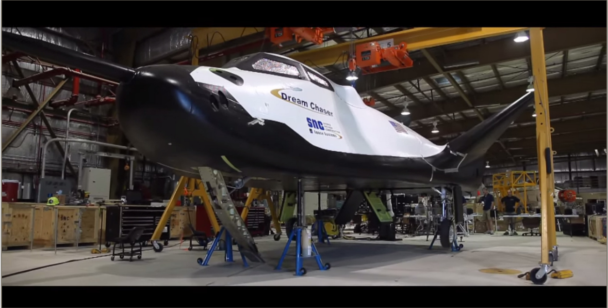
SNC's Commercial Dream Chaser atmospheric test vehicle under construction. Credit: Sierra Nevada Corporation (SNC)
