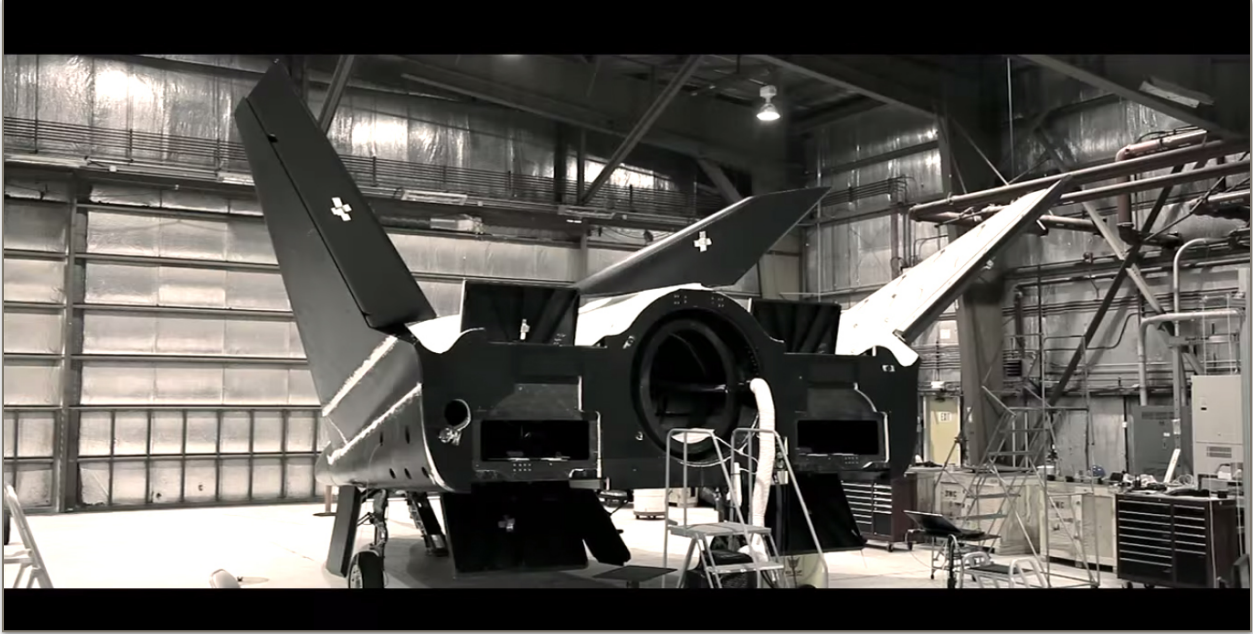
SNC's commercial Dream Chaser test vehicle under construction. Credit: Sierra Nevada Corporation (SNC)
